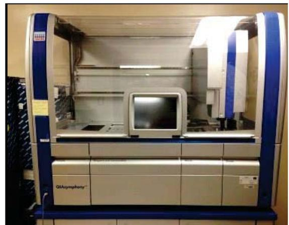
**Figure 7. Automated platform for DNA isolation**
